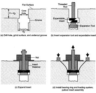
FIG. 2 Schematic of Procedure for Post-Installed Pullout Test
