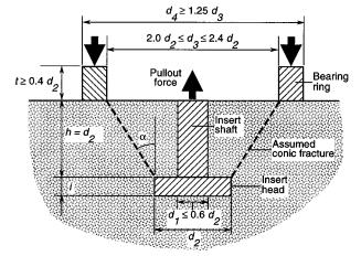
FIG. 1 Schematic Cross Section of Cast-in-Place Pullout Test
